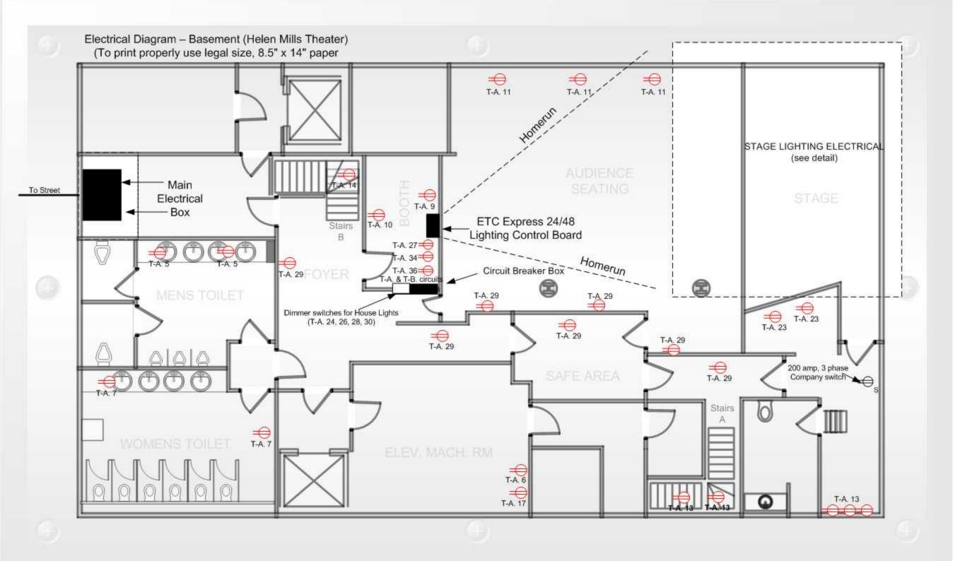
30 circuits from Lighting Wall Panel circuited into 30 dimmers controlled by ETC Express 24/28 lighting control board
